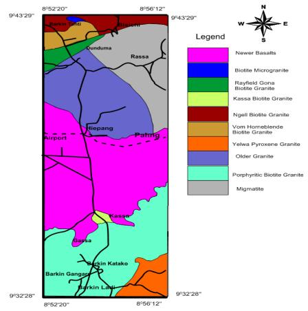
Fig. 2. Map Of The Study Area Showing The Different Lithologic Units
